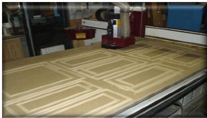
CNC Routers are used to create contoured edges, corners and 3D profiles in preparation for 3D Lamination
